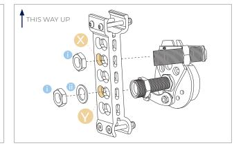
5 Slide drum brake kit bolts through holes 😣 and 💟
